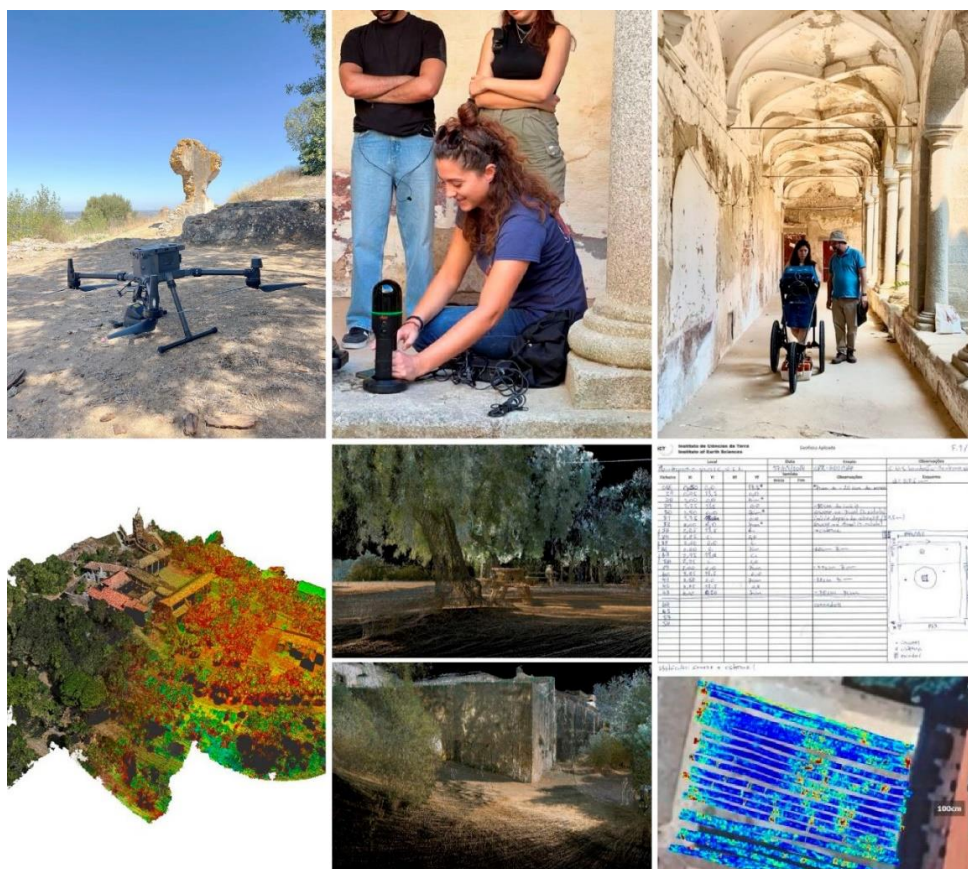
Figure 2. Digital surveys techniques for aerial, terrestrial and underground documentation. Equipments: Matrice 350 RTK with ZENMUSE L2, Leica BLK2GO, Ground Penetrating Radar (top, from left to right); 3D point cloud from aerial laser scanning, point cloud from terrestrial laser scanning, revealing of underground data (bottom, from left to right). ©Rolando Volzone, 2024.
